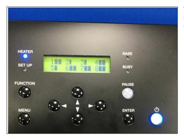
The ink indicator on the control panel displays one or two bars for the remaining ink level and lists numbers for each color instead of the actual color.
