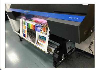
The take-up system, which comes standard with the TrueVIS VG-640, enables multiple jobs to be readily collected onto a core facilitating unattended print runs.
